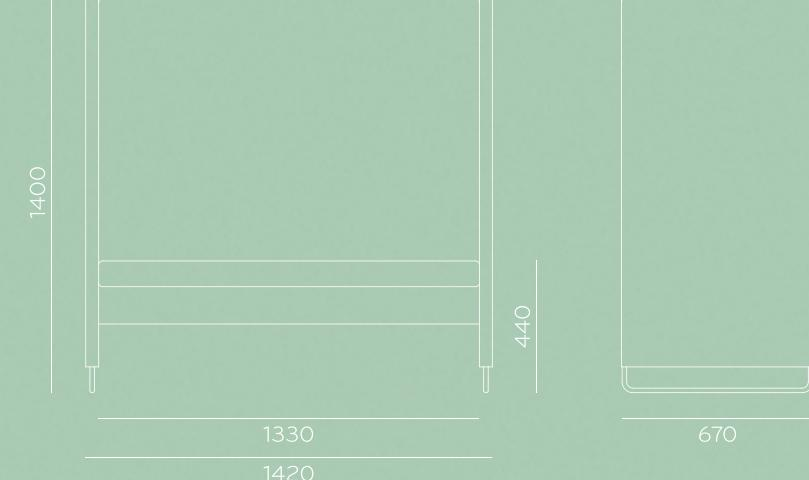
**Materials and Technologies:** fire-retardant polyurethane foam with variable density seat, steel frame. **Finishes:** upholstered with fabric or eco-leather. Black or white powder coated frame matched with the zip colour. **Options:** two seats or one seat sofa. Back side available in two different heights.
